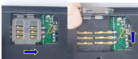
3 Put the SIM card into the holder, and turn the foil right and fasten it in place.
