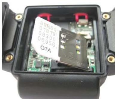
5.1.3 Insert the SIM card into the holder, press the foil down and put the battery in place.
