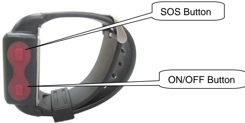
**NOTE:**As for ON/OFF Button,keep pressing 3 seconds is ON/OFF the tracker;while keep pressing 1 second is switch to displaying Latitude&Longitude.it displays Time,Date,Day and Battery in 30 seconds later automatically.
